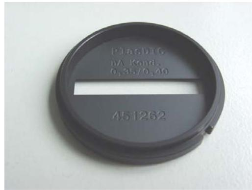
**Figure 5:** PlasDIC slider and slit diaphragm
